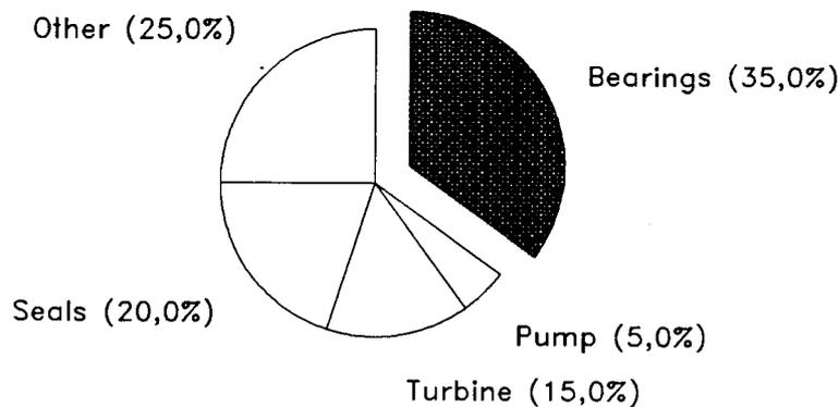
Figure 2 : Failure Mode Allocation for the VULCAIN LH2 Turbopump
