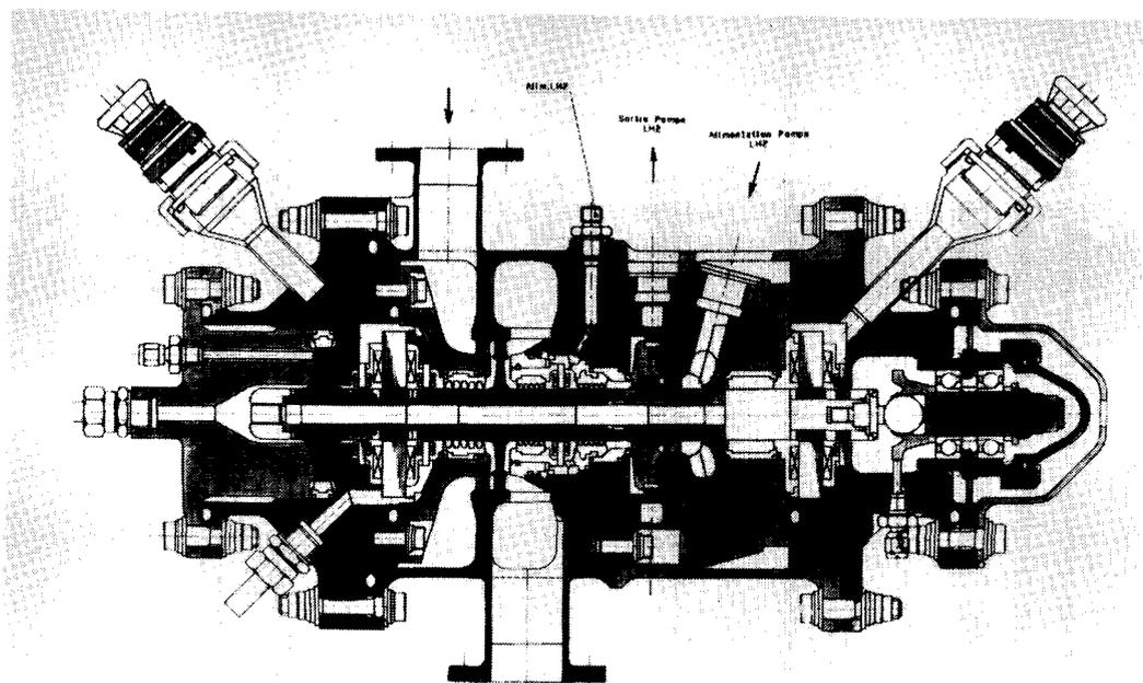
Figure 8. Turbomachine Design for AMB Qualification
