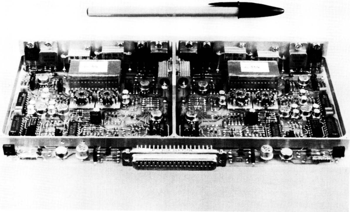
Figure 7. PC Board Prototype for Space-rated Power Amplifiers
