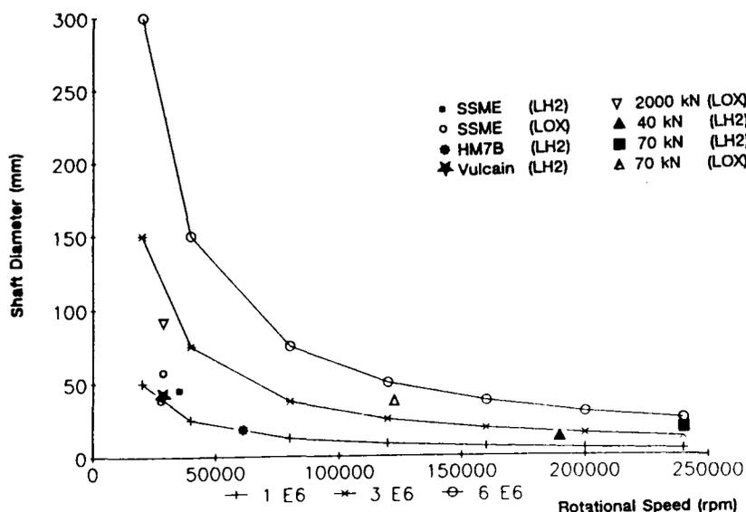
Figure 1 : Bearing D.N. Values for various T/P Designs
