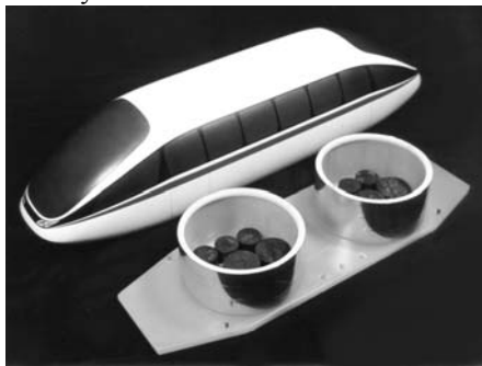
FIGURE 7 Demonstrator of linear transport system with SMBs of the joint Chinese German research project [9]).
