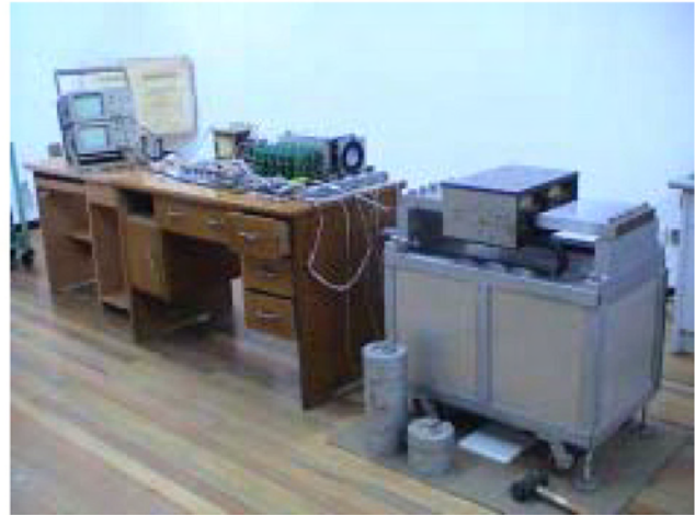
FIGURE 2 Experimental rig of working platform supported with AMG
