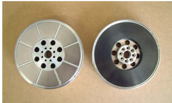
FIGURE 4: Rotor disks with 8 permanent magnets
