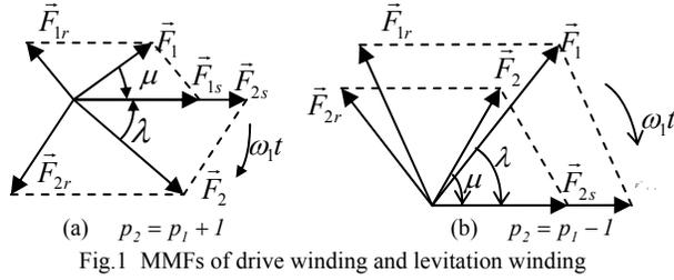
Fig.1 MMFs of drive winding and levitation winding
