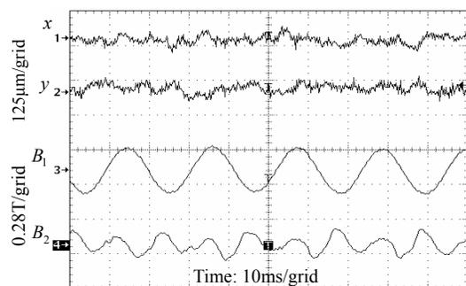
Fig.5 Waveforms of the independent levitated subsystem
