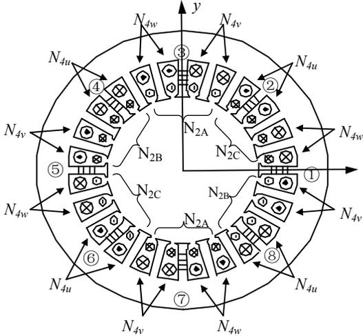
Fig.3 Stator winding arrangement in a motor prototype
