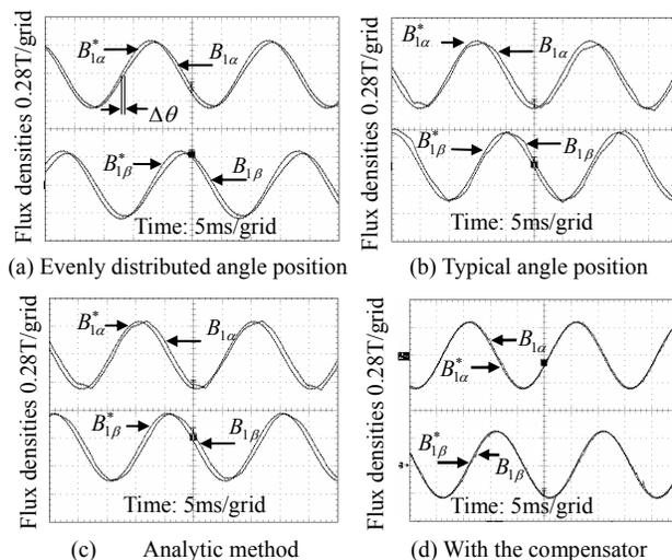
Fig.4 Waveforms of the air-gap flux densities of the drive winding
