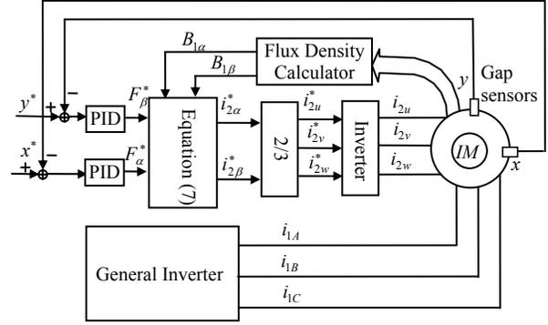
Fig.2 An independent control system of the levitation winding of bearingless induction motors
