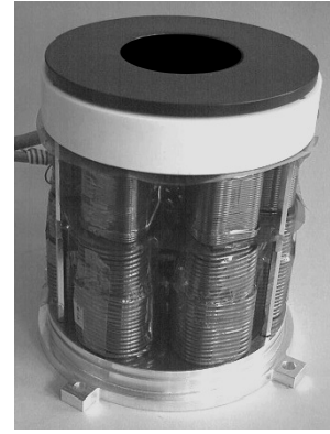
PICTURE 1: 4kW bearingless slice Motor with six slots
