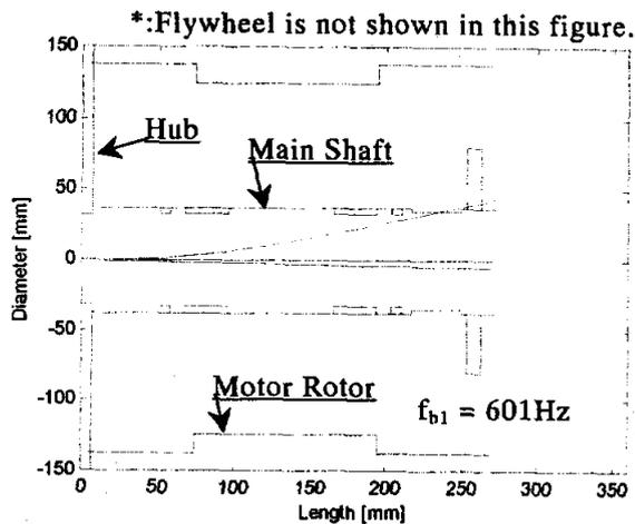
FIGURE 6: Analysis result of first bending mode frequency ( $f_{b1}=601\text{Hz}$ )
