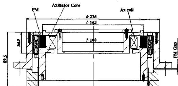
FIGURE 4: PM biased AxStator
