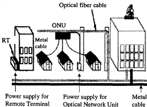
FIGURE 1 : Typical telephone network [1]
