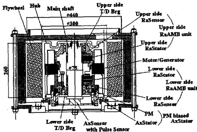
FIGURE 5: Schematic drawing of ComFESS
