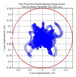
**FIGURE 5:** Displacement orbit at non-thrust end radial position sensor throughout the test
