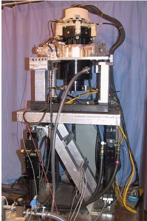
**FIGURE 3:** Flywheel battery system mounted on terrain simulator
