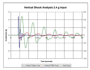
**FIGURE 9:** 3-dof analysis of axial shock test showing input, FWB response, and rel. displacement
