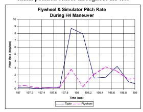
**FIGURE 6:** Simulator table and FWB response to 150% of maximum expected inputs (deg/sec)
