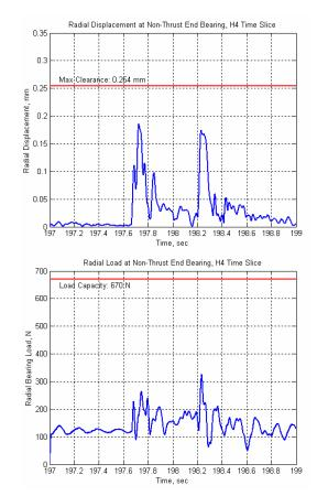
**FIGURE 7:** Non-thrust end bearing radial position (top) and radial loads (bottom) during maneuver H4
