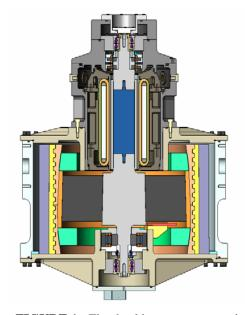
**FIGURE 1:** Flywheel battery cross-section
