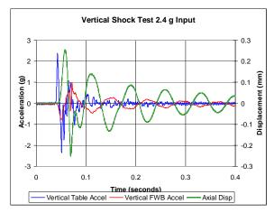
**FIGURE 8:** Axial shock test results showing 2.4 g input, FWB response, and relative rot/hsg displacement
