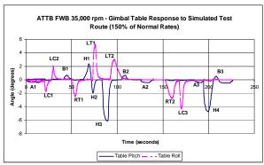
**FIGURE 4:** Terrain simulator table motion, 150% of maximum expected inputs
