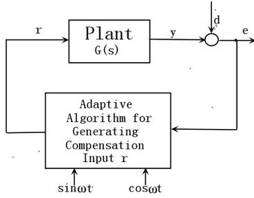
**FIGURE 1:** Block diagram of the control system rejecting periodic disturbance
