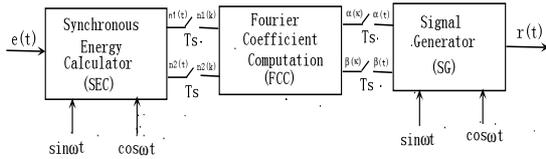
**FIGURE 2:** Block diagram of adaptive algorithm for internally generating reference signal
