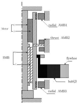
FIGURE 6: Cross-sectional view of outer rotor type flywheel
