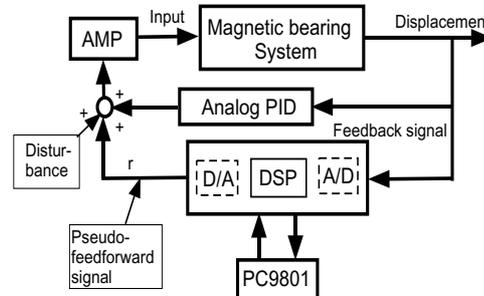
FIGURE 8: Block diagram for control system
