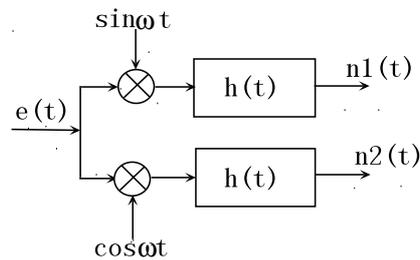
**FIGURE 3:** Details of the block SEC of **FIGURE 2**
