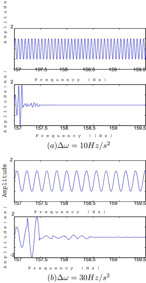
FIGURE 5: Displacement attenuation results for different frequency change rate.
