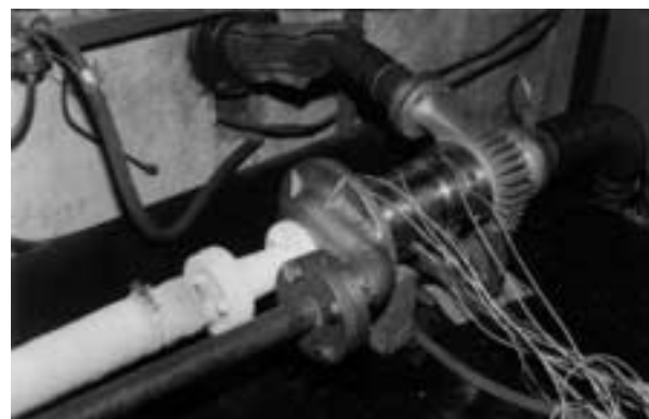
FIGURE 9 150M 3 oxygen gas turbo expander in experiment running.
