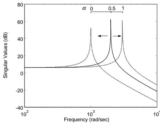
Figure 2 Vertex shaping filters (---) and linear interpolation (—)
