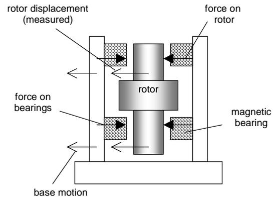
**Figure 3 Schematic diagram of experimental system**
