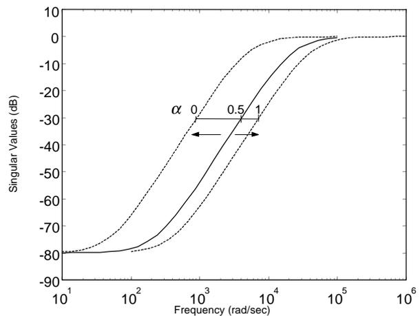
**Figure 6 Vertex shaping filters for design 2  $W_c$  (---) and linear interpolation (—)**
