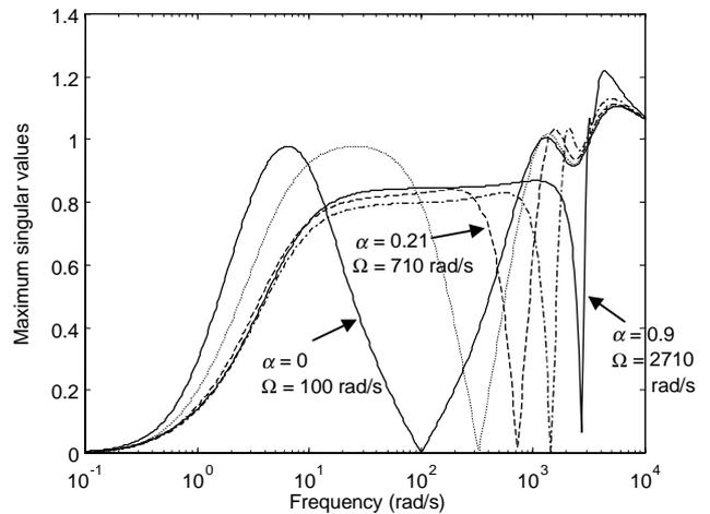
**Figure 5 Maximum singular values of sensitivity function for various rotational frequencies. Minima are collocated with rotational frequency**
