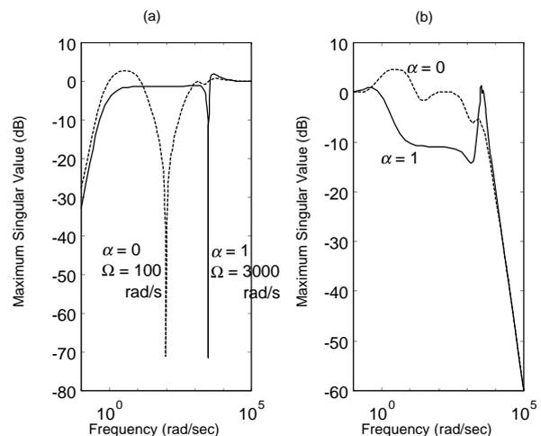
**Figure 4 Performance and robustness of the vertex systems for design 1: Maximum singular values of (a) sensitivity function (b) inverse sensitivity function**
