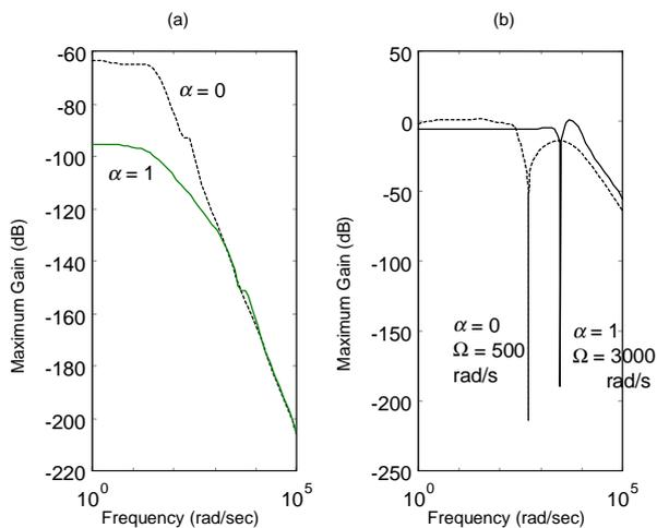
**Figure 8** Maximum RMS gain of the vertex systems for design 3 from rotor direct forcing input to (a) rotor displacements (b) bearing force
