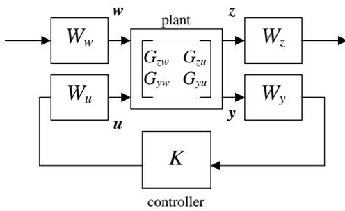
Figure 1 Closed loop system with shaping filters
