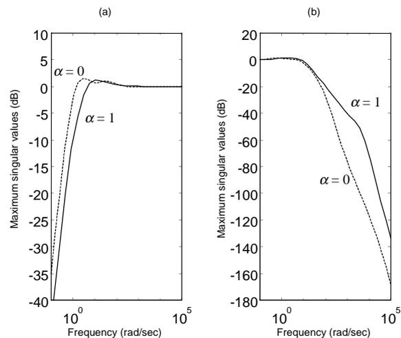
**Figure 7 Performance and robustness of vertex systems for design 2: Maximum singular values of (a) sensitivity function (b) inverse sensitivity function**
