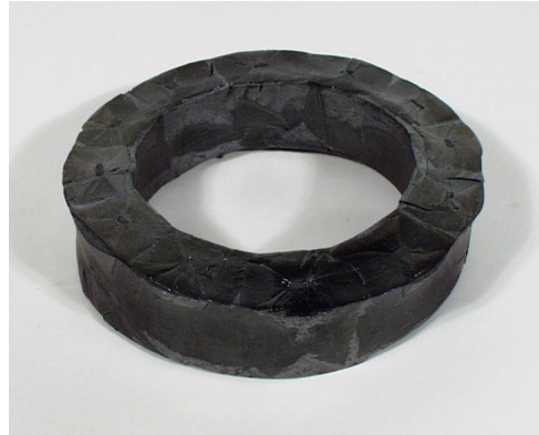
FIGURE 5: Multi-seeding melt-textured ring shaped HTSC [2]
