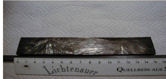
FIGURE 2: YBCO plate with 5 and 10 cm single domain structures grown without seeding in 80 hours
