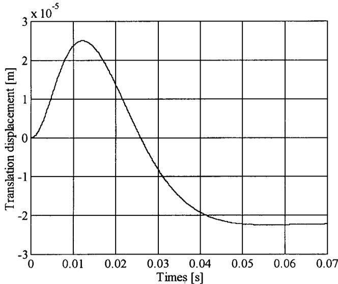
Figure 3. Rotor displacement in bearing plane to the step excitation of translation mode.
