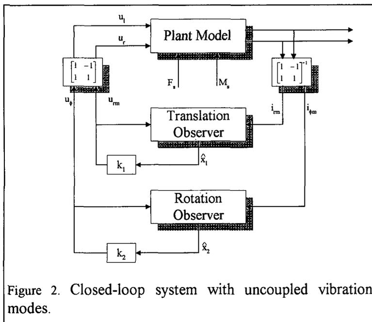
Figure 2. Closed-loop system with uncoupled vibration modes.
