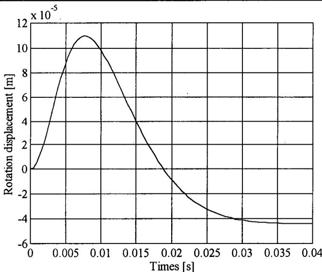
Figure 4. Rotor displacement in bearing plane to the step excitation of rotation mode for  $\Omega = 0$  [rad/s].
