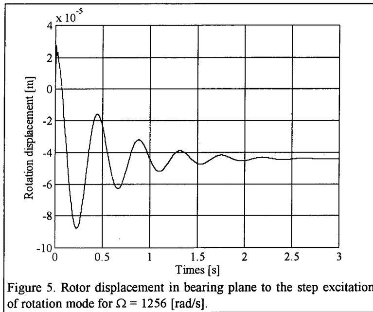
$= 0$  [rad/s] and in Figure 5 for  $\Omega = 1256$  [rad/s] = 12000 [rev/min]. We see that gyroscopic effects strongly influence the closed-loop dynamics. It was found the closed-loop system is unstable for angular velocities crossing the value  $\Omega = 1865$  [rad/s] = 17820 [rev/min]. If we reduce the values of the observer poles the system is unstable for lower angular velocity.
