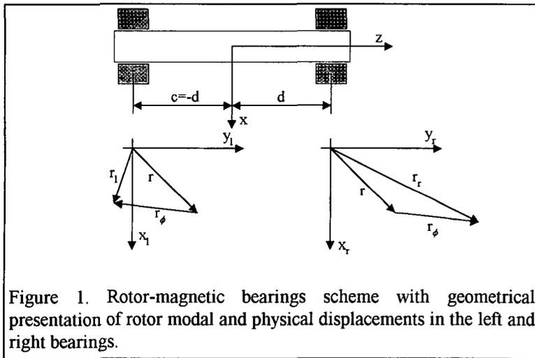
To simplify the consideration we assume that rotor mass centre has equal distance  $|c| = |d|$  from both bearings as it is seen in Fig.1. It is useful to change co-ordinate  $\phi$  by the co-ordinate  $r_\phi = z\phi$ . In the case  $z = d$  it is  $r_\phi = d\phi$  and this co-ordinate is located in the plane of right bearing. Modal displacements can be expressed by the rotor displacements in the bearing planes:
