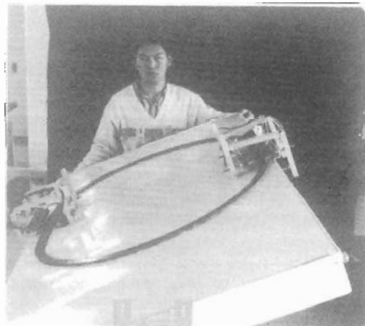
FIGURE 1: The Sm-Co loop. The whole apparatus is designed to be turned upside down for the hanging travel(see also Fig.12).
