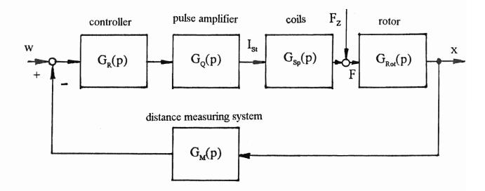
Distance measuring system: 20 V/mm, inductive-, capacitive- or eddy-current-measuring system Controller: PID-structure, analog
