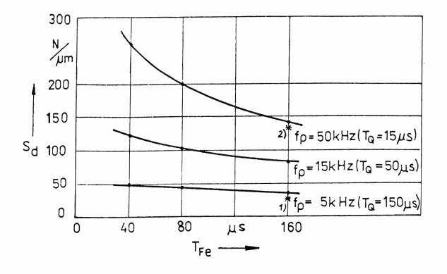
Fig. 3: Influence of the time constants  $T_{O}$  and  $T_{Fe}$  on the maximal achievable stiffness
