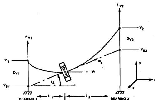
Figure 1: Flexible Shaft Definitions
