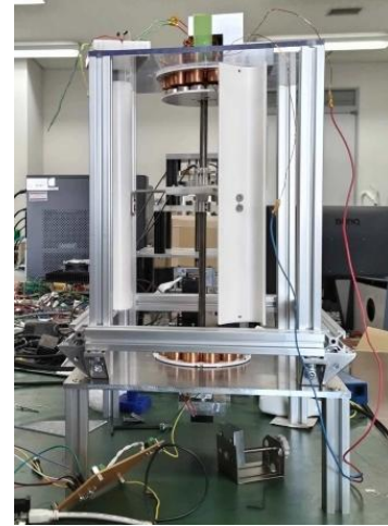
Fig. 2 Maglev vertical axis windmill.
