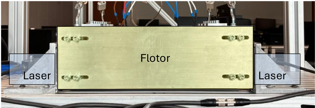
Fig. 4 Side view of the test bench. The flotor is suspended by hooks almost without friction and can move left and right. The lasers measure the flotor position differentially.
