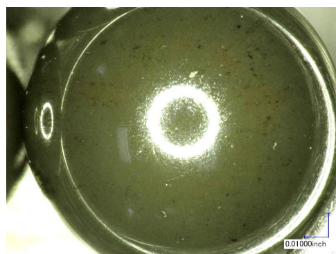
Fig. 12. Showing a ceramic ball from the inlet, inboard backup bearing (from Set2) after 100 drops
