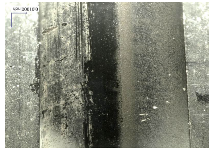
Fig. 10b. Photo of inlet, outboard backup bearing (from Set2) showing inner ring raceway after 100 drops.
