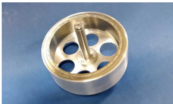
Fig. 2 Rotor of the proposed motor with smooth inner surface to be used as eddy-current sensor target. Outer diameter of the yoke is 79.3 mm, and axial length of the yoke is 18 mm.
