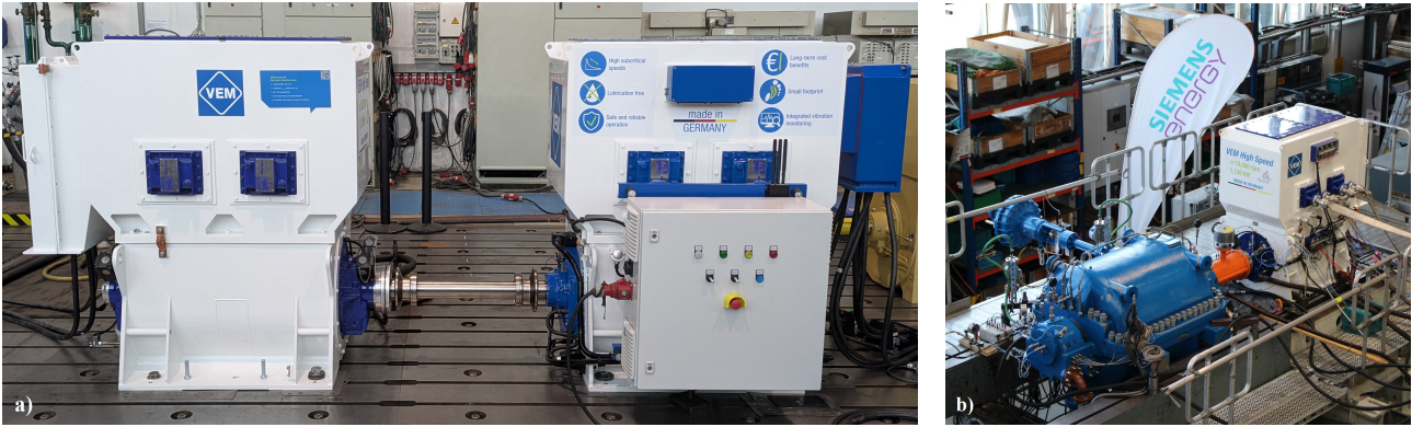
Figure 1 a) High-speed prototype motors (left: sleeve bearings, right: magnetic bearings) coupled with membrane-coupling, attached control cabinet with SpinDrive Magma X8000 MBC Controller for remote servicing b) Prototype with sleeve bearings coupled with turbo compressor in SEC test field © Siemens Energy, 2024 —Siemens Energy is a trademark licensed by Siemens AG.
