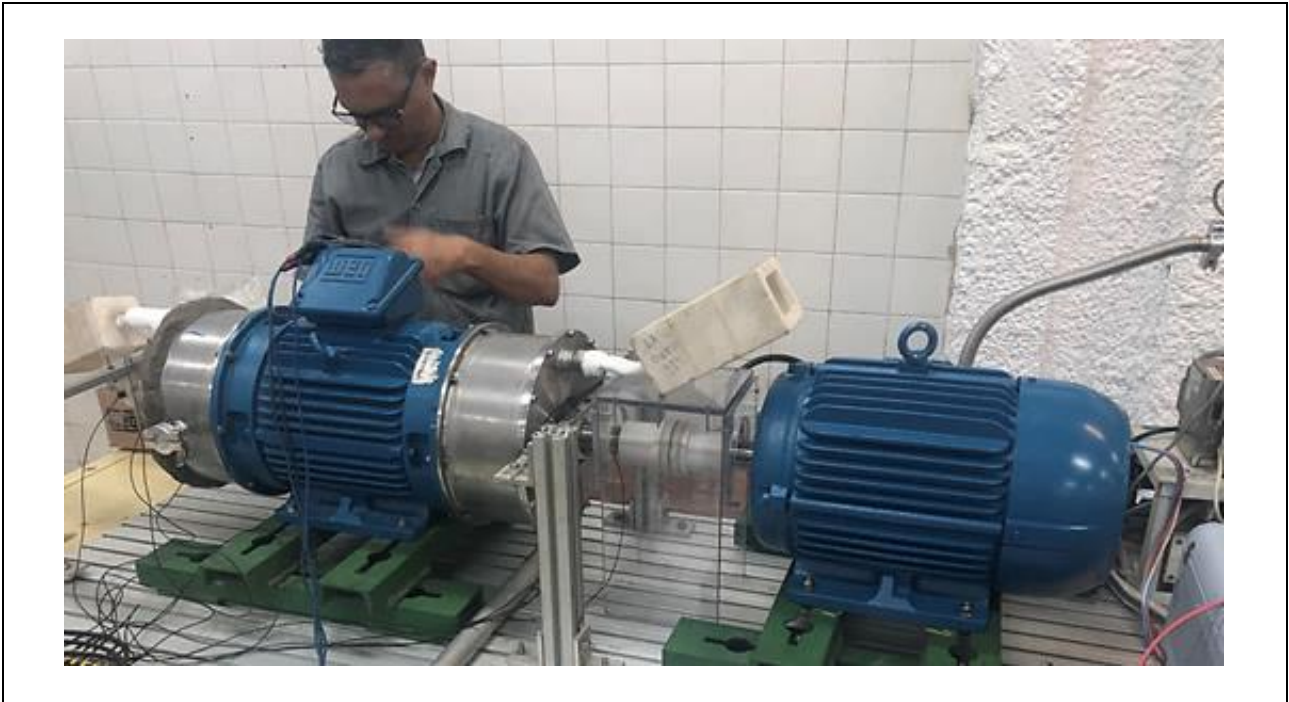
Fig. 7 Test bench showing the left electric machine supported by two PSMBs (PSMB 1 and PSMB 2), and the right machine (load machine) using a magnetic coupling.
