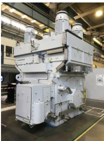
Figure 7 Induction motor 16MW@9000rpm on AMBs.
