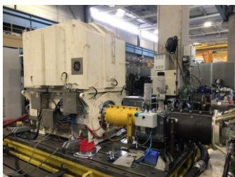
Figure 25 Testbench motor on AMB (on left) with thrust bearing gear (on right).
