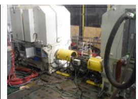
Figure 19 Back-to-back test arrangement.
