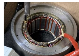
Figure 28 Testbench motor active magnetic bearing actuator.
