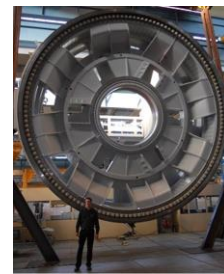
Figure 33 6MW@11rpm PM generator
