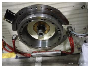
Figure 26 Testbench motor magnetic bearing integration.
