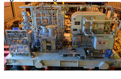
Figure 13 6.9MW-13200rpm off-shore export compression Service.
