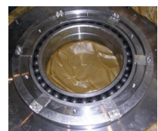
Figure 11 Ceramic landing bearing.
