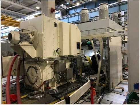
Figure 29 Rotor heat test arrangement (Testbench motor side).
