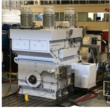
Figure 30 Rotor heat test arrangement (16MW Motor side).
