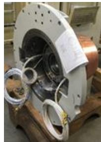
Figure 8 Active magnetic bearing integration for easy maintenance.
