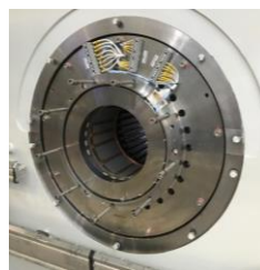
Figure 9 Non driven end active magnetic bearing.
