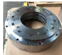
Figure 10 Landing bearing system.
