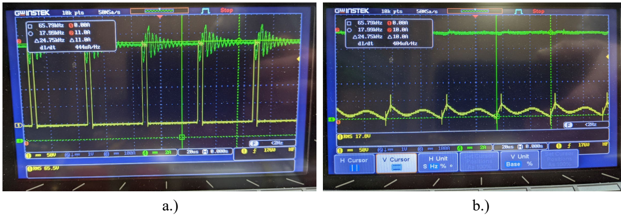
Figure 9. Measured voltage (yellow) and current (green) on the output of the amplifier without the filter (a) and with the filter (b). The DC output current component was 11.0A without the filter and 10.0A with the filter.
