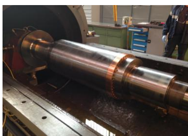
Figure 12 - HSEM Fully laminated rotor with AMBs
