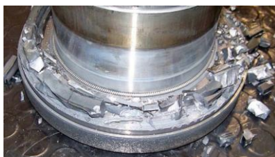
Figure 5 - Dry Gas Seal Catastrophic Failure
