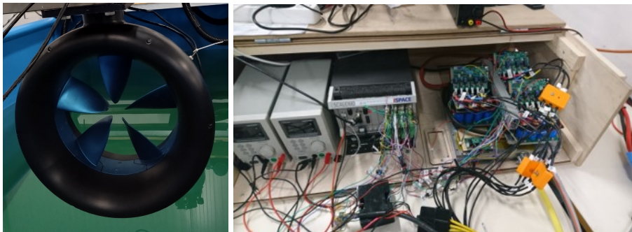
Figure 5: 20 kW hubless rim-driven thruster and control setup
