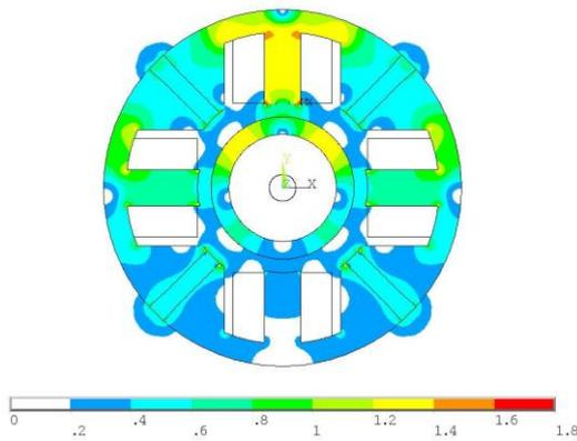
Figure 12 Flux density (Control current: 2 A).
