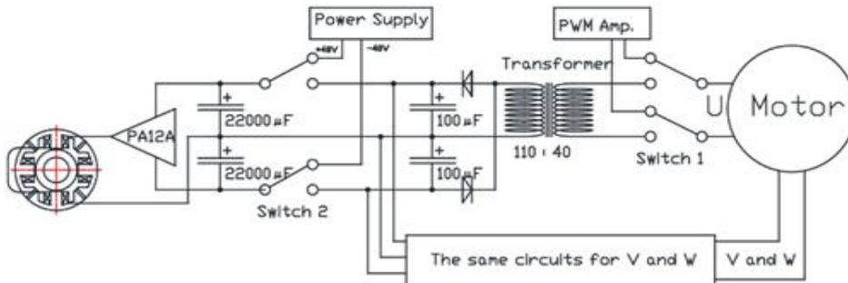
Figure 20 Regenerative circuit from motor to AMB.
