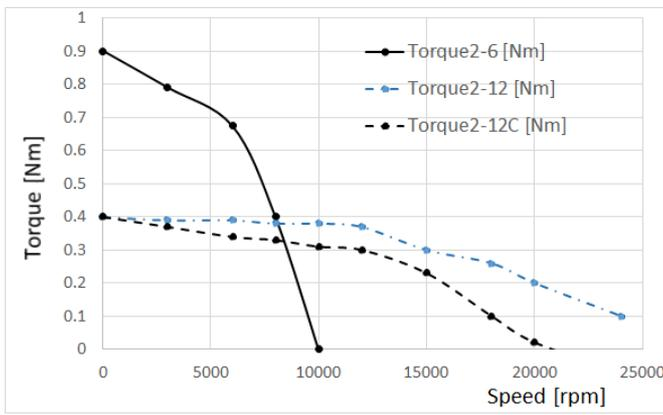
Figure 3 Torque versus speed curves (supply voltage: 72 V).
