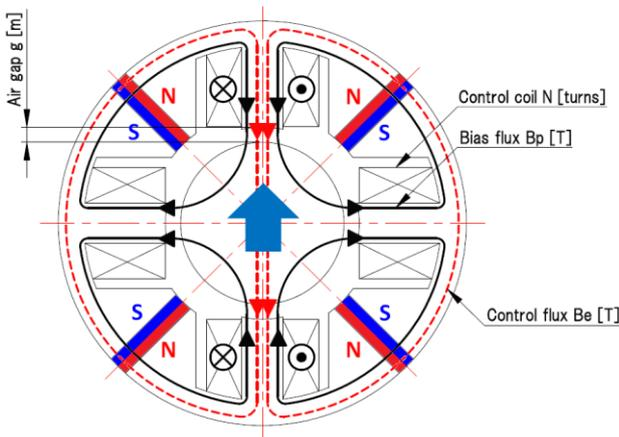
Figure 8 Operating principle of HB type magnetic bearing.
