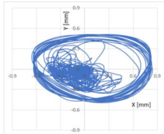
Figure 22 Orbital x-y trajectory after power shut down.
