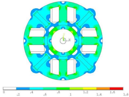
Figure 11 Flux density (Control current: 0 A).
