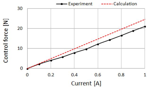
Figure 13 Force property of original magnetic bearing.
