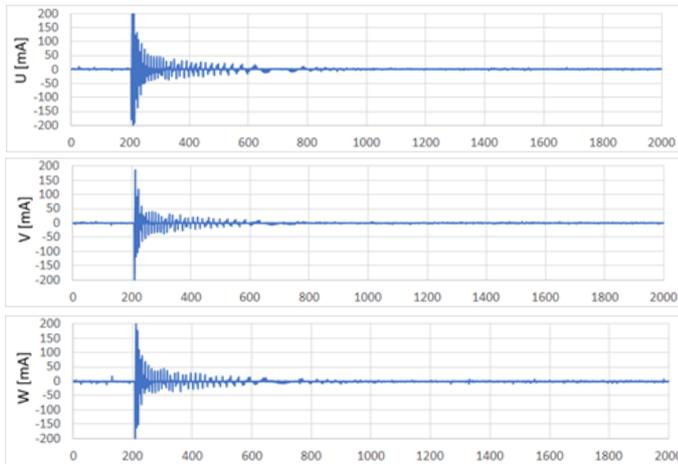
Figure 21 Regenerated currents of U, V, W phases [mA] versus time [ms].
