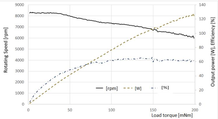
Figure 7 Torque versus speed curves (supply voltage: 72 V).
