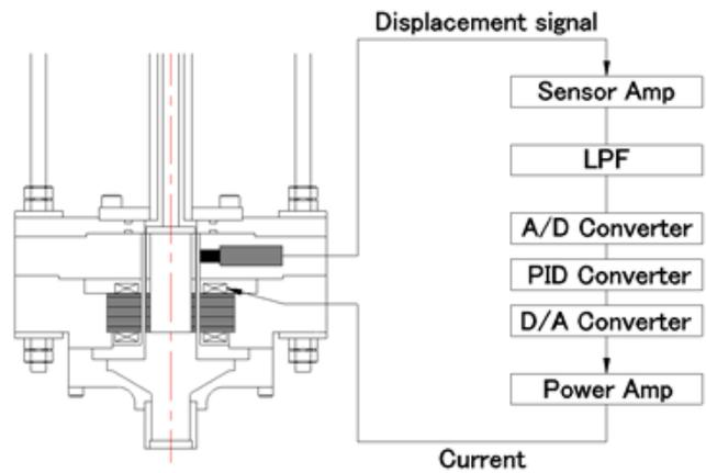
Figure 9 Magnetically supported pump and AMB controller.
