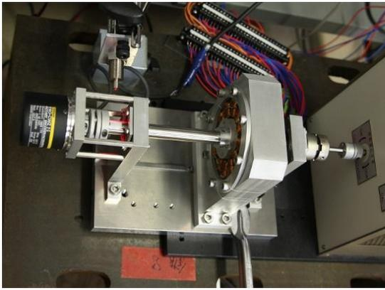
Figure 6 Motor is tested using motor analyzer.
