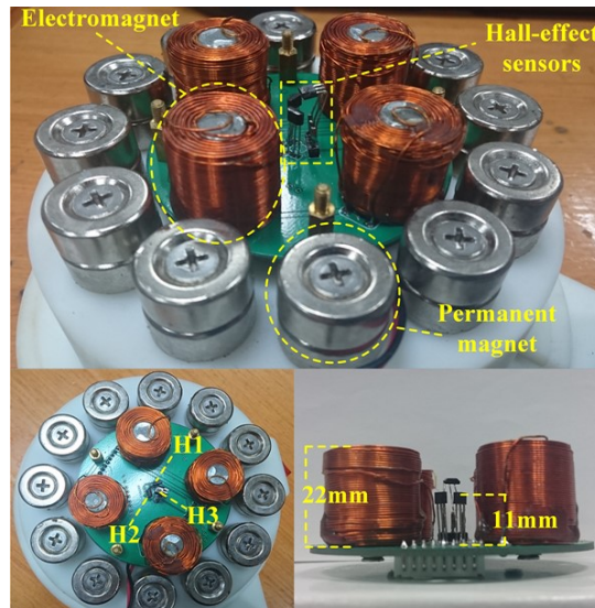
Figure 4: The laying position of the Hall sensors in the experimental device
