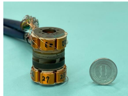
Figure 2: Developed ultra-compact double stator self-bearing motor.
