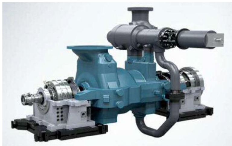
Figure 4 10MW feedwater pump on AMB installed in a fossil fuel power plant. Image: courtesy of Siemens (Turbinenwerk Görlitz)
