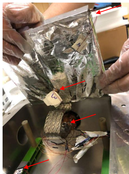
Figure 6. Temperature sensor distribution inside the cryostat.
