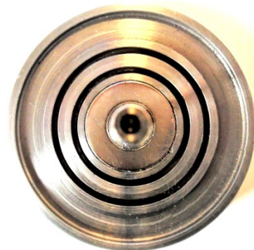
Figure 13. Manufactured armature of the HAMB in a form of the disc.
