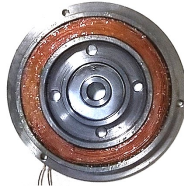
Figure 12. Manufactured top actuator of the HAMB.
