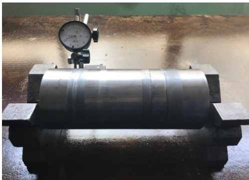
Figure 12. Test of radial circular run-out
