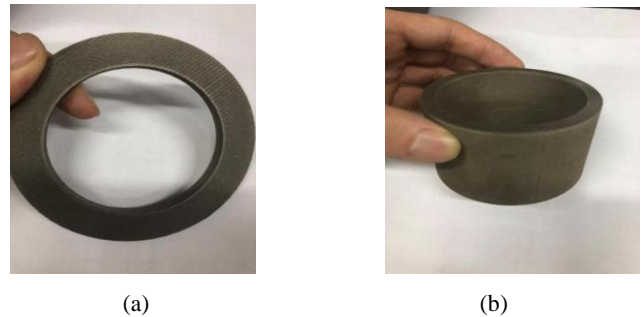
Figure 6. 3D printed thrust bush and lined bearing bush
