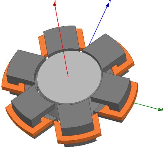
Figure 8. Concept with six bearing coils, opposite coils are wound with in opposing sense and are connected to same phase.
