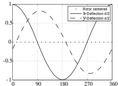
Figure 4. Normalized sum-flux through sensing coil in three distinct situations for an eccentricity of half the air gap width.
