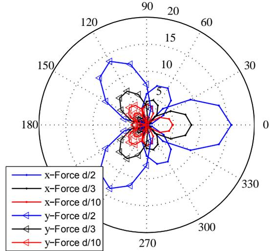
Figure 7. Disturbance forces in Newton in x- and y-direction over  $\varphi_{el}$  in degree in synchronous orbit for different eccentricity values in fractions of the air gap  $d$ .
