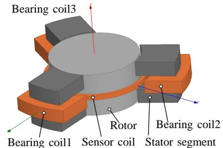
Figure 2. Concept demonstration system: 3-phase, 3-segment magnetic bearing
