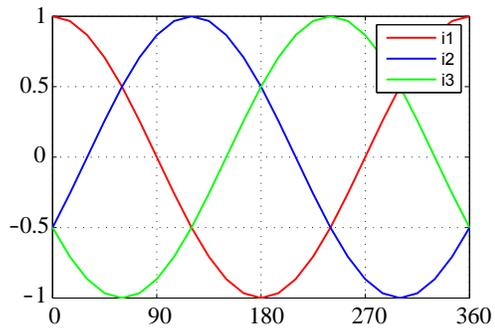
Figure 3. Normalized currents in three-phase system for non-deflected rotor.
