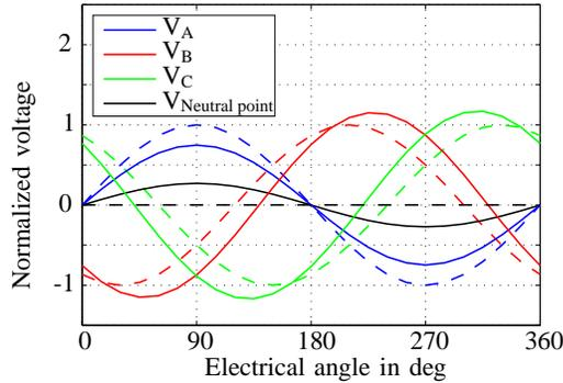
Figure 11. Principle of neutral point shift for reducing e.g. phase A voltage compared to non-shifted voltages (dashed)
