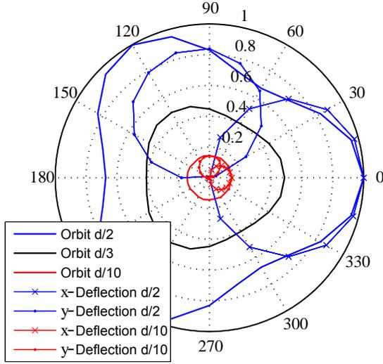
Figure 5. Normalized sum-flux through the sensing coil over  $\varphi_{el}$  in degree in case of an orbit synchronous to the electrical system ( $\varphi_{mech} = \varphi_{el}$ ) and two stationary rotor deflections in x- and y-direction (i.e.  $\varphi_{mech} = 0^\circ$  or  $90^\circ$ , respectively) for different eccentricity values in fractions of the air gap  $d$ .
