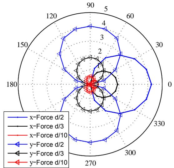
Figure 10. Disturbance forces in x- and y-direction on the rotor in Newton over  $\varphi_{el}$  in degree in synchronous orbit for different excentricity values in fractions of the air gap  $d$  for the 6-coil system.
