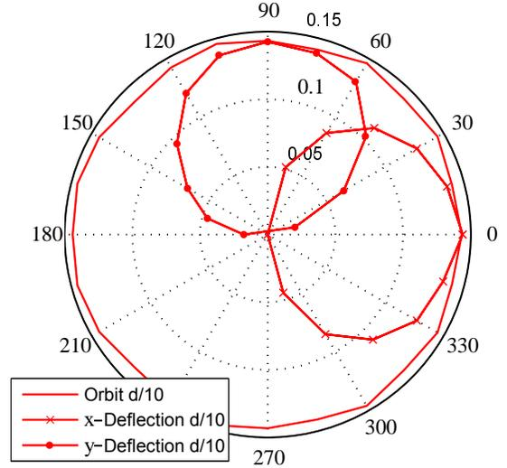
Figure 6. Zoom of Figure 5 showing the sum-flux over  $\varphi_{el}$  in degree in synchronous orbit, x- and y-deflection (i.e.  $\varphi_{mech} = 0^\circ$  or  $90^\circ$ , respectively) for  $\varepsilon = \frac{d}{10}$ .
