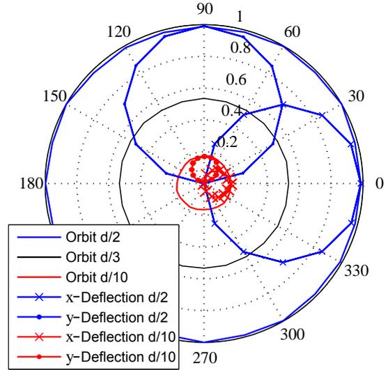
Figure 9. 6-coil sum-flux through the sensing coil over  $\varphi_{el}$  in degree in case of an orbit synchronous to the electrical system ( $\varphi_{mech} = \varphi_{el}$ ) and two stationary rotor deflections in x- and y-direction (i.e.  $\varphi_{mech} = 0^\circ$  or  $90^\circ$ , respectively) for different excentricity values in fractions of the air gap  $d$ .
