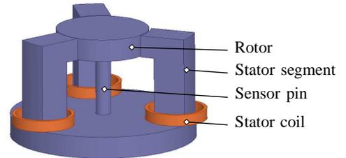
Figure 1. Concept of sum-flux detection in [5] with a sensor pin carrying a dedicated flux sensor.
