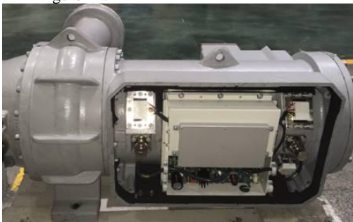
Figure 14. Application of new power amplifier in the magnetic levitation centrifuge
