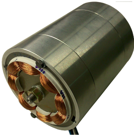
Figure 9. Eight-pole AMB with bias coils for self-sensing control applied to a high speed synchronous reluctance machine.
