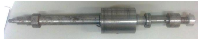
Figure 2. Shaft with laminated silicon steel rotor [3].
