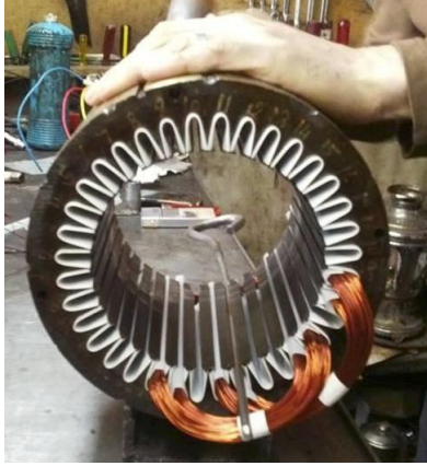
Figure 3. Stator of a three-phase induction motor with 36 slots [7].
