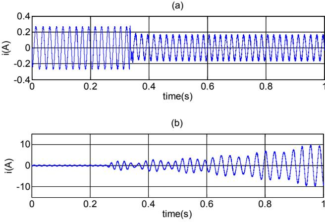
Figure 5. Simulation verification result when the rotation speed is 50Hz. (a) current vibration of AMB control system with compensation angle  $\theta_k = \pi$ . (b) current vibration of AMB control system with compensation angle  $\theta_k = 0$ .
