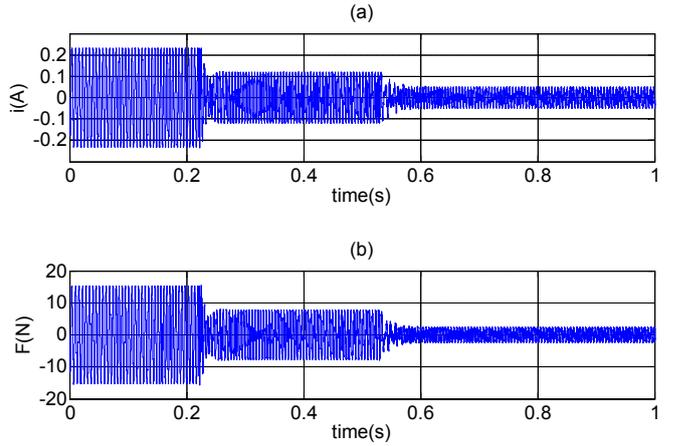
Figure 8. Comparison of suppression effect between the method with current suppression only and the novel SRF-based method at 12000r/min. (a) control current after two method applied. (b) vibration force after two method applied.
