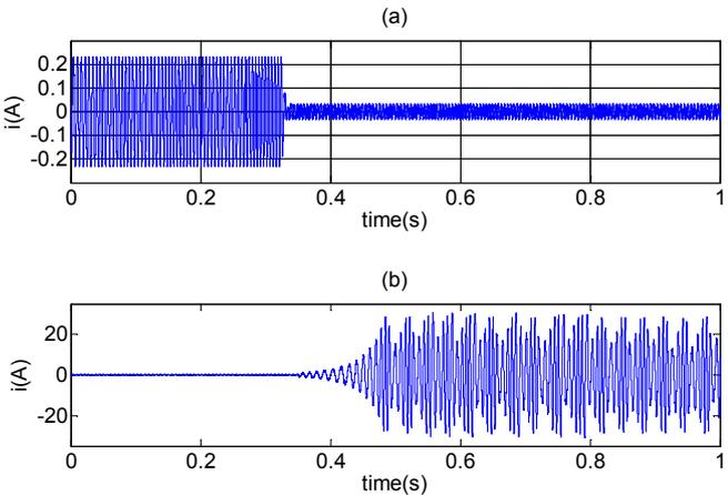
Figure 7. Simulation verification result when the rotation speed is 200Hz. (a) current vibration of AMB control system with compensation angle  $\theta_k = 0$ . (b) current vibration of AMB control system with compensation angle  $\theta_k = \pi/2$ .
