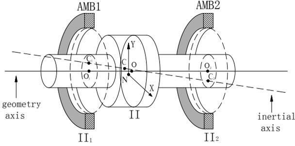
Figure 1. The basic structure diagram of magnetic suspended rotor with mass unbalance .
