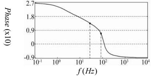
Figure 4. The phase frequency response curve of sensitivity function.
