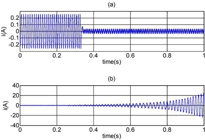
Figure 6. Simulation verification result when the rotation speed is 100Hz. (a) current vibration of AMB control system with compensation angle  $\theta_k = \pi/2$ . (b) current vibration of AMB control system with compensation angle  $\theta_k = 0$ .
