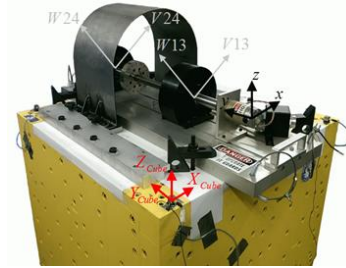
Figure 4. Experimental test rig on the hydraulic shaker
