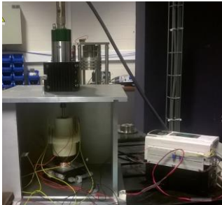
Figure 7. Picture of the test bench to operate the prototype in quasi-static conditions, with an external motor to drive the rotor.
