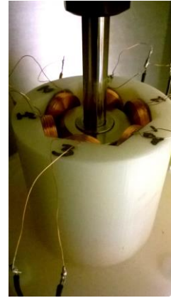
Figure 5. Picture of the centering heteropolar electrodynamic bearing prototype, investigated for its torque generation and self-centering capacities
