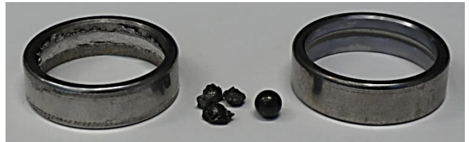
Figure 21. Bearing outer rings and ceramic balls. Left: the failed backup bearing components from the second test series. Right: functional components from the first test series.
