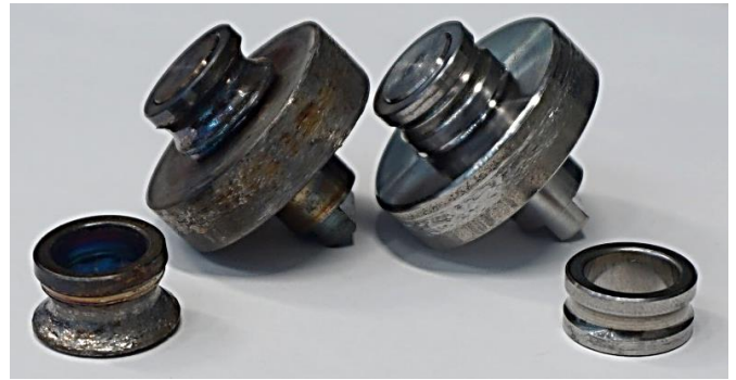
Figure 20. Bearing inner rings and BBU rollers. Left: the failed backup bearing components after the second test series. Right: functional components after the first test series.
