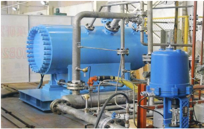
Figure 2. Fuel ball blowers (helium compressors) for HTR-PM.
