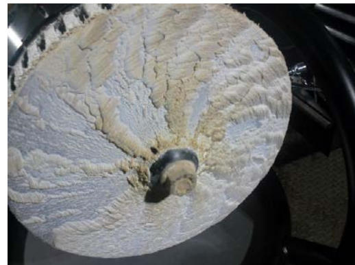
Fig. 2. Atomizer wheel with uneven buildup.
