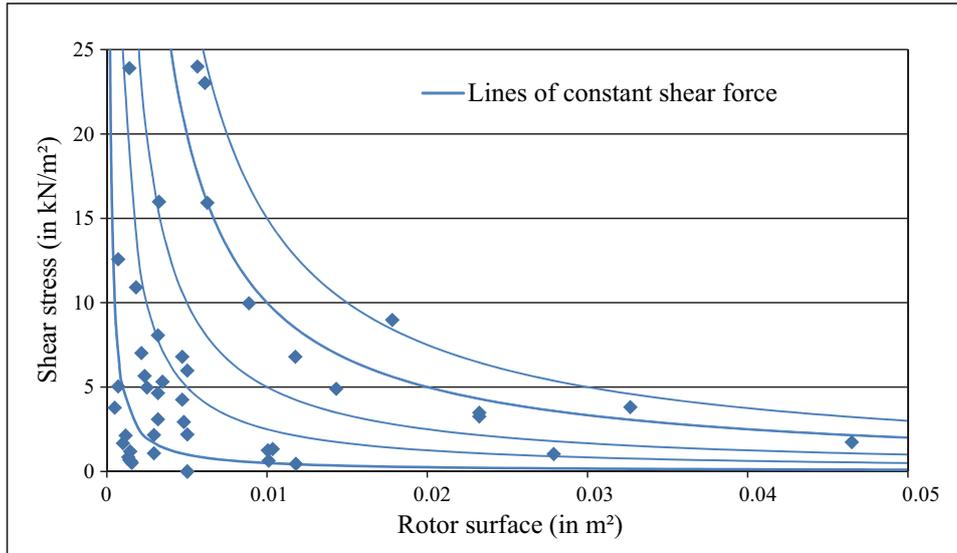
Figure 4: Shear stress plot of reported bearingless slice motors.
