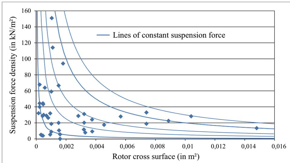
Figure 5: Suspension force density plot.
