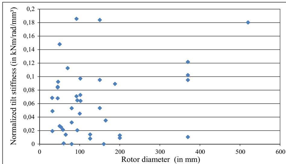
Figure 6: Comparison of the passive tilt stiffness values.
