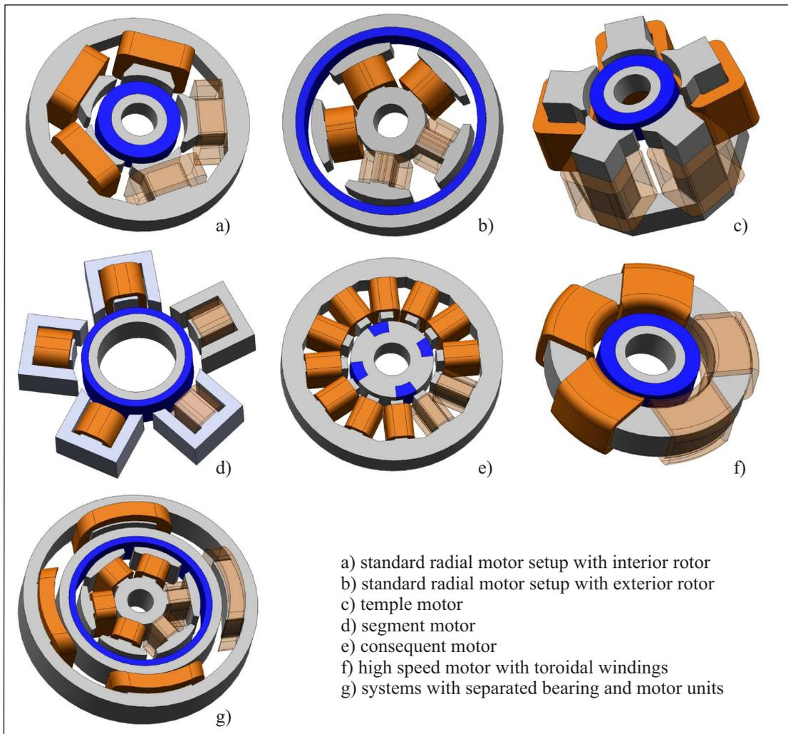
Figure 1: Different implemented bearingless slice motor topologies.
