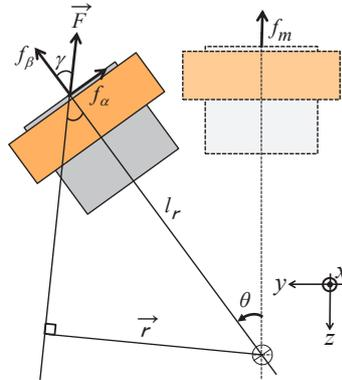
Fig. 5 Torque acting on the carrier
