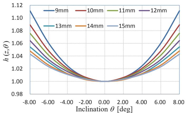
Fig. 4 Calculation result of attractive force fluctuation ratio
