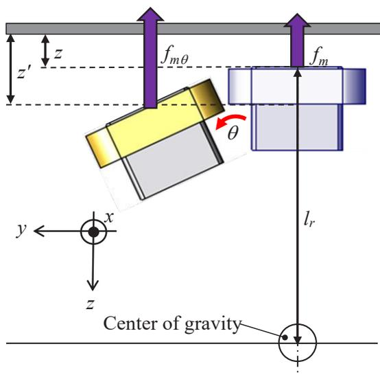
Fig. 3 Model of rolling motion
