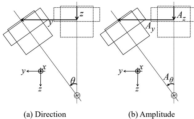
Fig. 2 Separating of rolling motion
