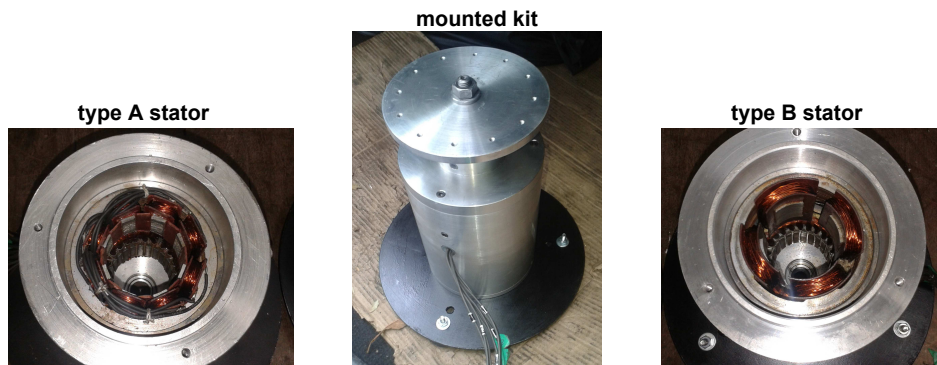
Fig. 3 Top view of prototypes A, in the left and B in the right; notice the 8 “poles” in type A, and only 4 “poles” in type B. A mounted kit is shown in the center, with a vertical rotor inserted in one of the carcasses.
