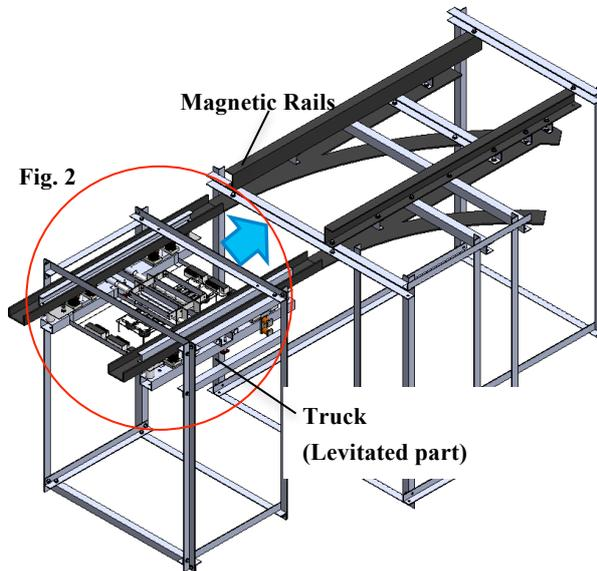
Fig. 1 Diagram of the equipment.
