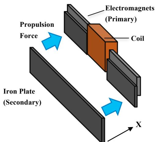
Fig. 3 Diagram of one unit of the LSRM.
