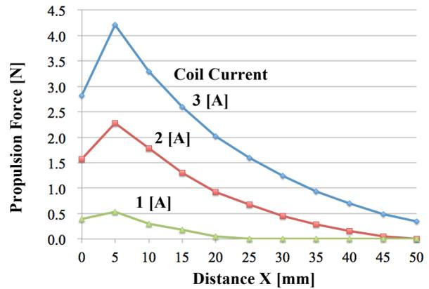
**Fig. 9 Static experiment results of LSRM at thickness of iron core 18 mm.**
