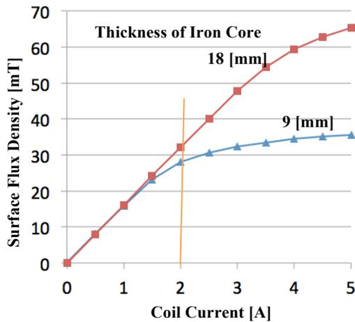
**Fig. 8 Experimental results of the electromagnet.**
