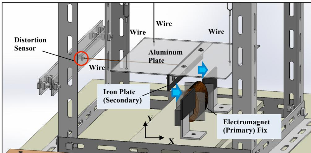
Fig. 5 Diagram of the static experimental apparatus.
