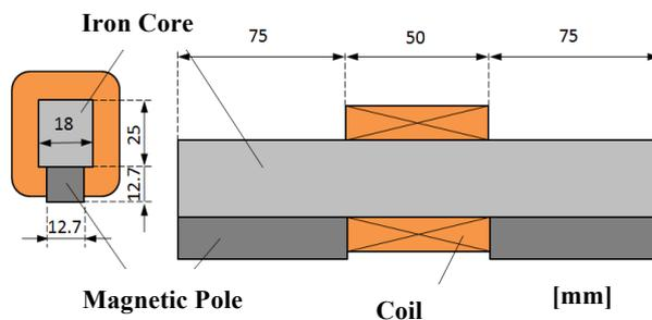
Fig. 6 Design drawings of the electromagnet.
