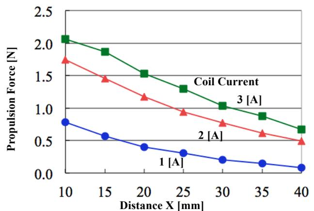
Fig. 4 Static experiment results of LSRM with 9-mm thick iron core.
