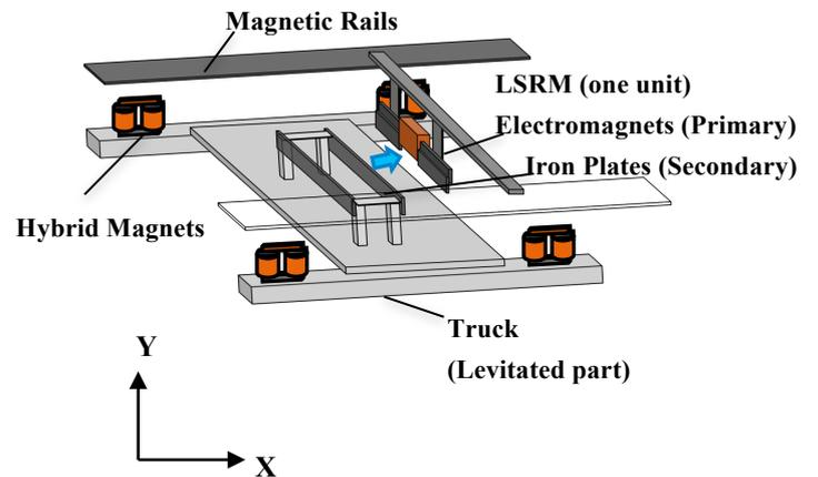
Fig. 2 Structure of the LSRM and levitation part.
