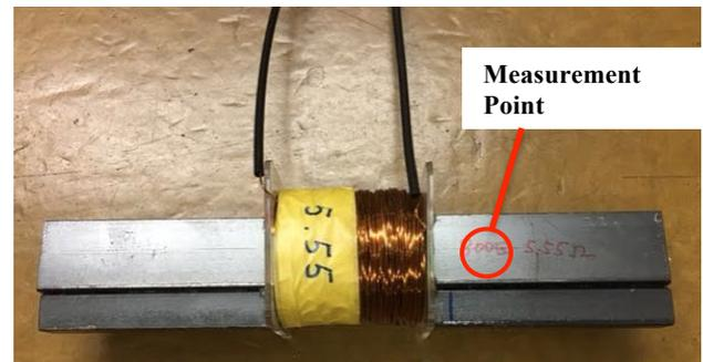
Fig. 7 Photo of the electromagnet.
