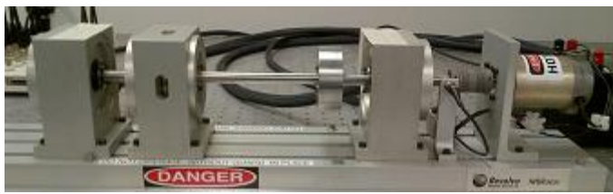
Fig. 2 AMB test rig A) photograph, and B) basic dimensions. The test rig has a steel shaft supported by two radial AMBs and one thrust AMB manufactured by SKF. The rotor is driven by a DC electric motor via a flexible coupling. There is one disk between the bearings and each AMB has a target rotor. The TD bearings are rolling element type and are to the immediate outside of each radial AMB rotor.
